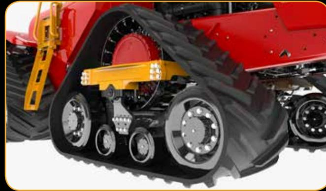
The DeltaTrack uses a positive drive system to reduce friction, heat, and wear. Track slippage is eliminated by interlocking track lugs into the drive wheel. The DeltaTrack keeps 6.5 lugs engaged with the drive wheel at all times to eliminate slippage between the track and drive wheel. The DeltaTrack uses the largest drive lugs available (8-1/2") in the industry to maximize operating life.
